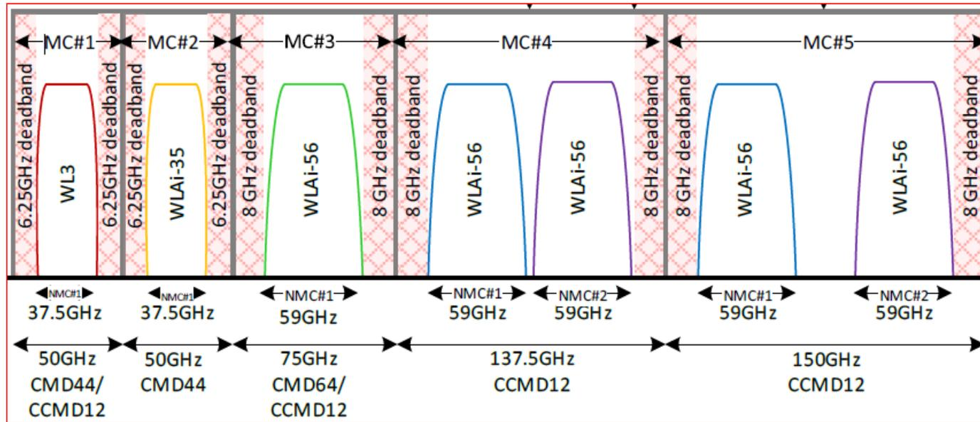
**Note:** Multiple NMC per MC are supported for optical channels between colourless directionless ROADMs on CCMD12. One control will not support Multiple NMC per MC provisioning, but the same will be supported under BP MCP 18.10 onwards.
