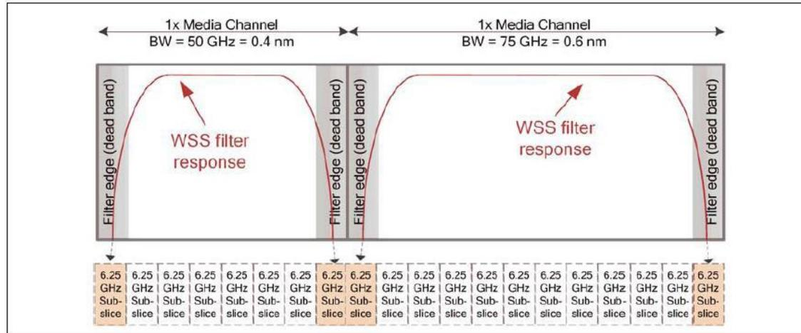
Telecom operator's current FixGrid Ciena 6500 based DWDM ROADM network operates on standard ITU 50GHz fixed spectrum grid. Current set of CMD44 filters deployed in the network are capable of supporting 88 optical channel per OMS section.
