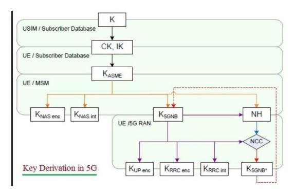
The Good news about EN-DC is that it works almost the same way the LTE-DC runs the concepts of Key Generation, Key Management, Ciphering and Integrity Protection are re-used from LTE – DC concept TS23.501 while the DRB <Data Radio Bearer Security> context is added with regard to 5G Core Network. For EN-DC security, new X2 Information Elements, "SgNB security Key" and "UE Security Capabilities" is newly defined.
