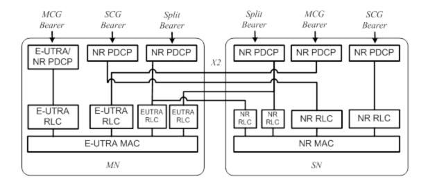
Here shows EN-DC bearers and PDCP termination points from Network side. MN is the master eNB and SN is the secondary gNB. If the PDCP/NR-PDCP is terminated in the MN, LTE security works, on the other hand, if the NR-PDCP is terminated in the SgNB, NR security covers. EEA is redefined as NEA, EIA is also
